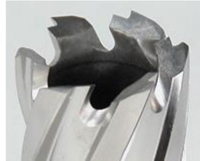
With their unique centerfree design, annular cutters cut only the periphery of the hole, ejecting the remaining center as a slug. These cutters produce reamed quality, burr-free holes in one operation, eliminating costly pilot holes and step drilling. Our cutters reduce torque and horsepower requirements by only cutting the periphery of the hole using the proper tooth geometry.
